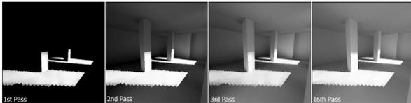
Figure 2: Shows how the radiosity technique spreads the radiance in each iteration (render by *H. Elias*).
