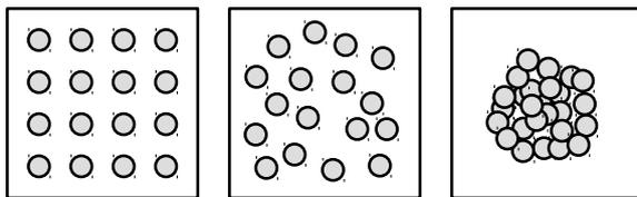
Figure 11: Visualization of *supersampling patterns* we’ve implemented: *grid*, *random*, and the *gaussian*. Another common technique is *jittering* (not shown).
