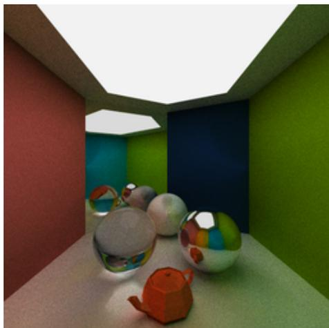
As expected the final results give less noise with more samples but at the cost of additional computation time. This also reduces aliasing and thus the jaggies which were presented earlier. The aliasing near the sources of light is especially bad at the start because it doesn't fall off as smoothly as the other surfaces in the scene. That is, it's a very sharp change in color, and it thus takes a lot of samples to blend it with the nearby colors.
