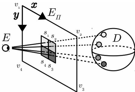
Figure 9: Intuition for *supersampling* anti-aliasing technique. Average the samples  $s_1, s_2, s_3, s_4$  to find the pixel’s expected color. Usually not four samples.
