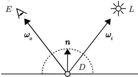
Figure 5: Diffuse ‘‘Lambertian’’ surface.
